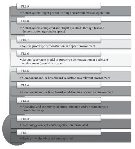
FIGURE 2.1 Technology readiness levels. (Courtesy of NASA.)
